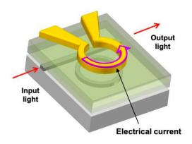
Perspective view of the device (not to scale). The electrical current in the metal coil is used to apply a radial magnetic field to synthetic magneto-optic garnet underneath. The silicon microring and the silicon waveguide, in the all-pass filter configuration, are visible through the transparent top-cladding.
