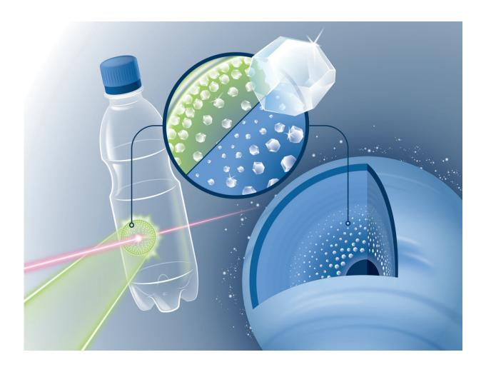
In the experiment, a thin sheet of simple PET plastic was shot at with a laser. The strong laser flashes that hit the foil-like material sample briefly heated it up to 6000 degrees Celsius and thus generated a shock wave that compressed the matter to millions of times the atmospheric pressure for a few nanoseconds. The scientists were able to determine that tiny diamonds, so-called nanodiamonds, formed under the extreme pressure. Credit: HZDR / Blaurock
