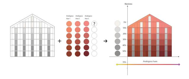
Here's a conceptualization of the pixelization method that could be used with different color solar panels on a pitch roof façade. Credit: *Solar Energy* (2021). DOI: 10.1016/j.solener.2021.06.079
