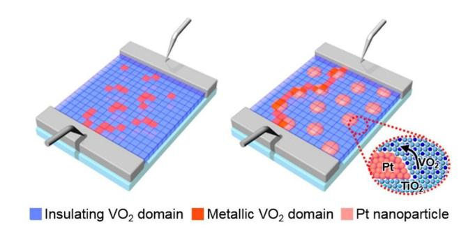
Schematic of the effect of the "stepping-stone" current flow formed via the platinum nanoparticles inserted in the thin phase-transition oxide film. Credit: POSTECH
