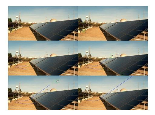
Argonne model detects moving objects (green boxes) and tracks their movements (blue lines). Non-bird objects (e.g., shadow and reflection) are filtered out prior to activity classification. Credit: (Image by Argonne National Laboratory).
