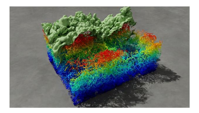
A section of a rising thermal wall plume reveals the intricate structure of eddies of air. Each tube represents a different turbulent vortex. Credit: Sivaramakrishnan Balachandar
