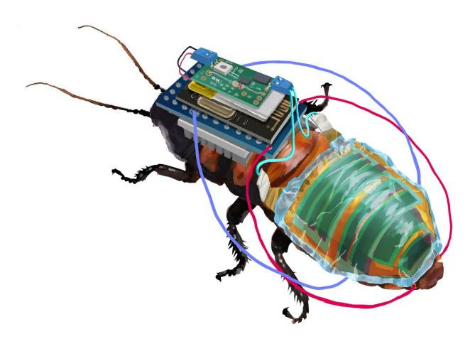
Researchers at RIKEN, Japan have created remote controlled cyborg cockroaches, equipped with a tiny wireless control module that is powered by a rechargeable battery attached to a solar cell. Credit: RIKEN
