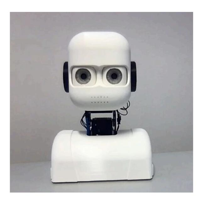
Epi the humanoid robot used by Krantz and his colleagues, is a humanoid robotics platform used for human-robot interaction experiments and cognitive
