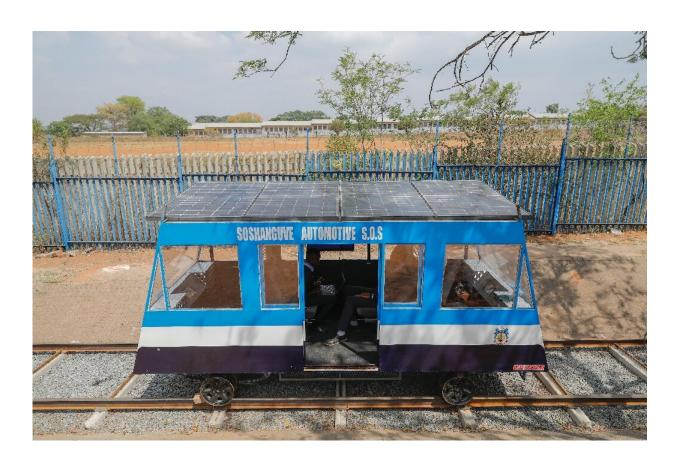
Photovoltaic panels fitted on rooftop, the blue-and-white train moves on an 18-metre long testing track in Soshanguve township.
