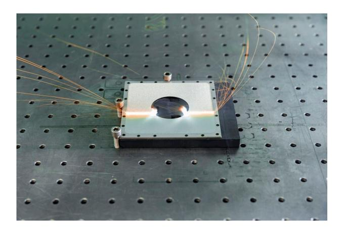
The laser blasting system precisely processes only the desired surfaces, consuming neither sand nor material for masking, thus saving hazardous and tape waste. Credit: René Jungnickel/Fraunhofer IWS
