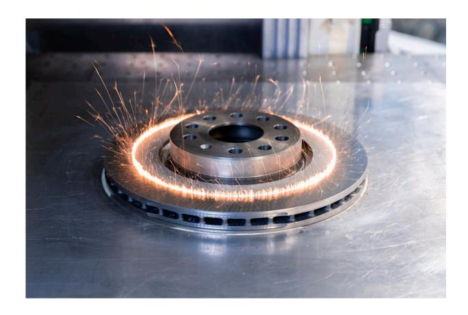
Sandblasting at the speed of light: Fraunhofer IWS uses high-energy light instead of sand grains to clean and roughen – for example the surface of brake discs. Credit: René Jungnickel/Fraunhofer IWS
