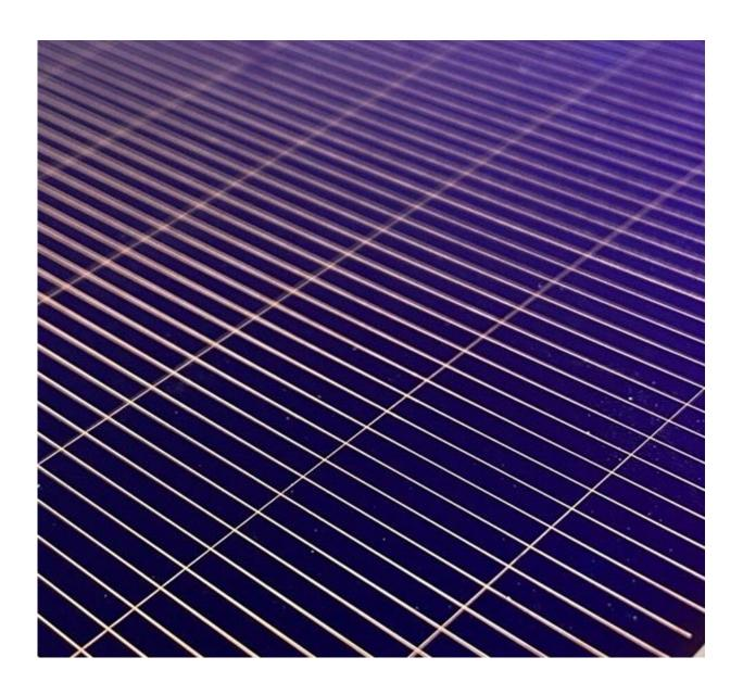
At just 19 micrometers in width, the copper contacts are extremely thin. As a
