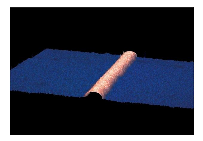
Three-dimensional confocal microscopy image of a copper contact produced using the laser-assisted process developed by PV2+. The even, semi-circular shape of the contact ensures a high level of electrical conductivity. Credit: PV2+
