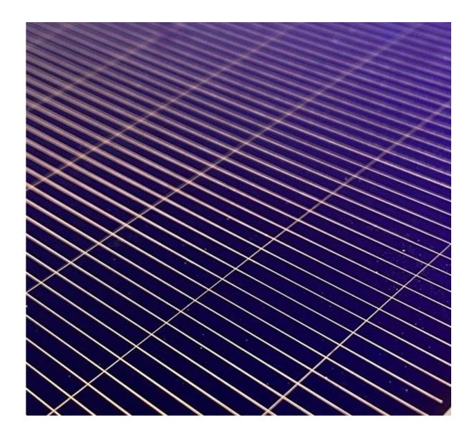
At just 19 micrometers in width, the copper contacts are extremely thin. As a
