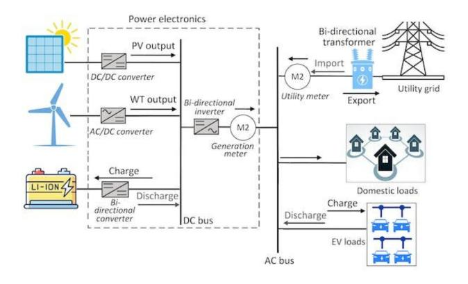
The modelled microgrid includes wind and solar power, a community battery and a fleet of electric vehicles. Author provided
