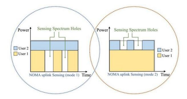
Schematic diagram of uplink hybrid IoT sensing scene and an illustration for frequency band occupancy status. Credit: SARI
