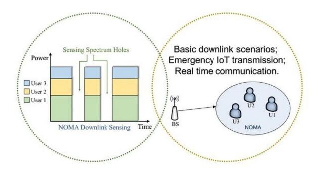
Schematic diagram of downlink hybrid IoT sensing scene and an illustration for frequency band occupancy status. Credit: SARI
