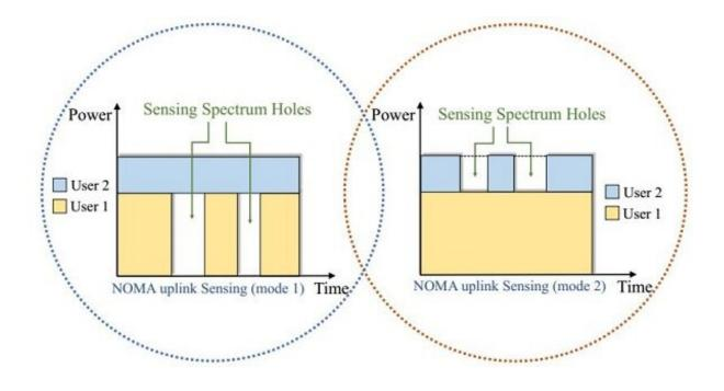
Schematic diagram of uplink hybrid IoT sensing scene and an illustration for frequency band occupancy status. Credit: SARI
