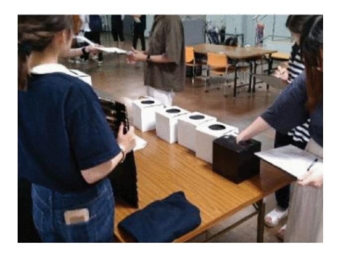
Experimental setup. A reference smartphone cover and smartphone covers with varying surface textures were placed in different boxes. Credit: Yoshihiko Kadoya
