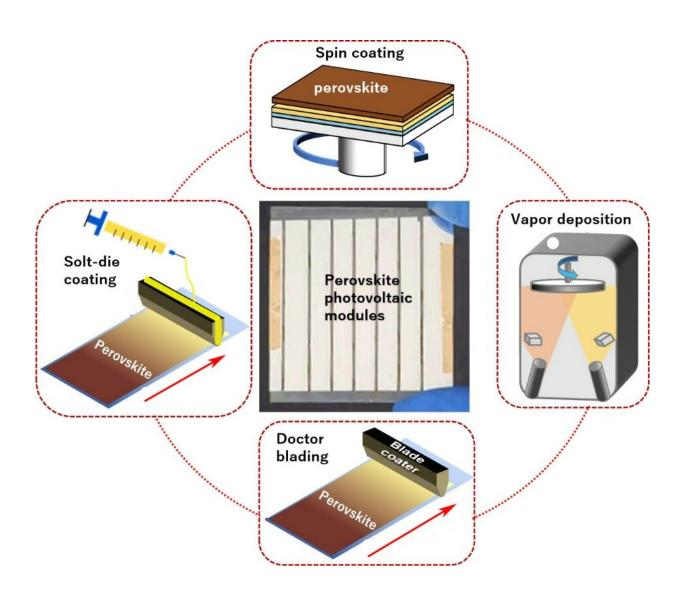
The research team summarized the advances of perovskite photovoltaic modules with particular attention paid to the coating methods, including spin coating, doctor blading, slot-die coating, spray coating, inkjet printing, soft-cover
