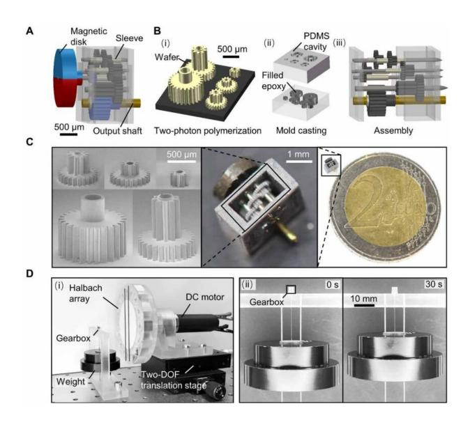
Design and performance of the magnetically actuated miniature gearbox for millimeter-scale magnetic actuators. Credit: *Science Robotics* (2022). DOI: 10.1126/scirobotics.abo4401
