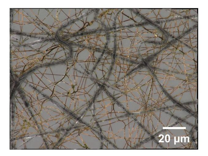
Magnified Confocal microscope image of the all-mesh thermistor. Credit: Chihiro Okutani, Shinshu University
