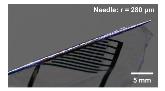
A photograph of the mesh thermistor wrapped around a needle. Credit: Modified from *Advanced Science* (2022). DOI: 10.1002/advs.202202312
