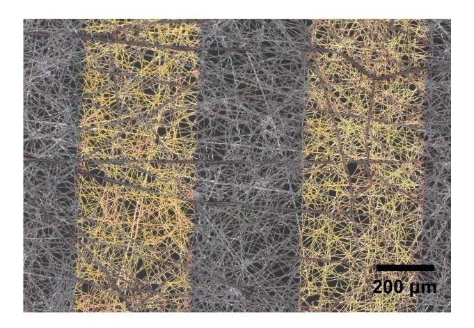
This photograph shows the structure of the ultrathin mesh-type polymer PTC thermistors used in wearable medical devices. There are many potential benefits to using mesh in this type of device. Credit: Chihiro Okutani, Shinshu University
