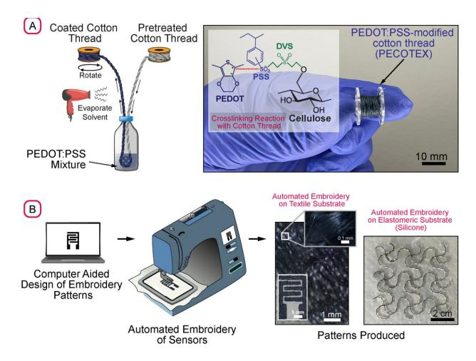
(a) Synthesis of PECOTEX and a photograph of the produced thread on a bobbin. Inset shows the chemical structure of the product; (b) Process for computerised embroidery of patterns using PECOTEX and 1 mm thick silicone substrates. Credit: Güder Research Group
