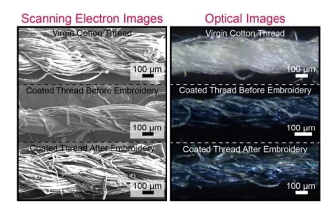
Scanning electron and optical micrographs of a cotton thread, PECOTEX, and PECOTEX after embroidery. Credit: Güder Research Group
