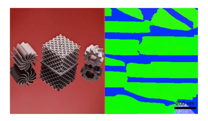
Through laser powder bed fusion, the discovered eutectic high-entropy alloy can be used to develop complex, nanolayered structures. Credit: Dr. Kelvin Xie
