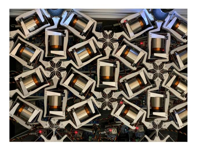
Photo of a mechanical neural network (MNN). Currently, the system is about the size of a microwave oven, but the researchers plan to simplify the MNN design so that thousands of the networks can be manufactured on the micro scale within 3D lattices for practical material applications. Credit: Flexible Research Group at UCLA
