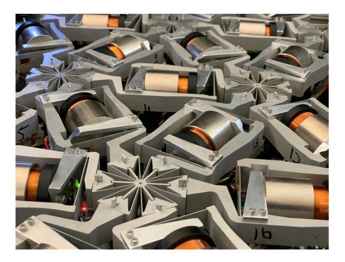
Photo of a mechanical neural network (MNN). Currently, the system is about the size of a microwave oven, but the researchers plan to simplify the MNN design so that thousands of the networks can be manufactured on the micro scale within 3D lattices for practical material applications. Credit: Flexible Research Group at UCLA
