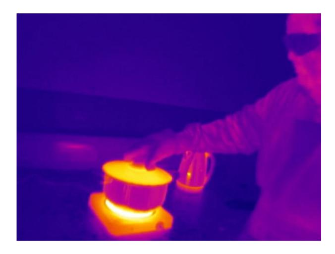
Heat dissipation shown by an infrared camera, lighter colour shows a higher temperature. Credit: Amin Al-Habaibeh, Author provided
