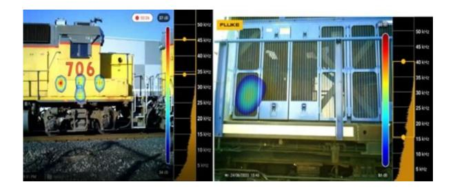
SwRI developed an automated compressed air leak detection system that can acoustically and visually detect and report air leaks on moving trains, indicated by spectral signatures in the photos. The team tested the proof-of-concept system on rail cars and trains at SwRI's Locomotive Technology Center in San Antonio. Credit: SwRI
