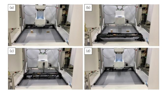
How the system actually works: (a) Initial state (b) Automatic cleaning toilet bowl cleans over the rim. The floor cleaning robot moves to the front of the toilet space. (c) The floor cleaning robot collects urine and debris scattered on the floor while also cleaning the sides of the toilet bowl. (d) Cleaning is complete. Credit: Tezuka et al.
