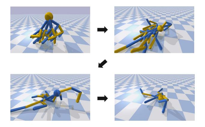
The evolution of a robot from a sufficiently complicated morphology to one more suitable for walking. Credit: Koike et al.
