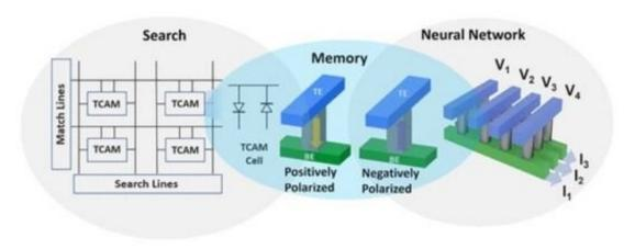
The transistor-free compute-in-memory architecture permits three computational tasks essential for AI applications: search, storage, and neural network operations. Credit: *Nano Letters* (2022). DOI: 10.1021/acs.nanolett.2c03169
