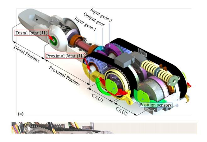
A sectional view of the CAD model of the finger (top) and the prototype antagonistic variable stiffness finger mechanism (bottom). Credit: Higher Education Press Limited Company
