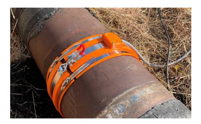
Southwest Research Institute (SwRI) has created the next generation of transducers that use ultrasonic guided wave technology to detect anomalies in pipes, enabling users to prevent leaks before they start. Credit: Southwest Research Institute
