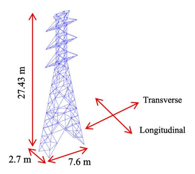
A schematic representation of the studied transmission tower illustrating the dimensions and main loading directions. Credit: *Earthquake Engineering & Structural Dynamics* (2022). DOI: 10.1002/eqe.3735
