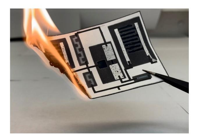
An electronic circuit printed on paper could be a more flexible and disposable option for single-use electronics. Credit: *ACS Applied Materials & Interfaces* (2022). DOI: 10.1021/acsami.2c13503
