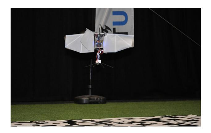
Flapping-wing robot controlling its attitude using this new principle. It is equipped with an artificial compound eye inspired by insects, which can perceive optical flow at a high frequency. Credit: Christophe De Wagter/TU Delft
