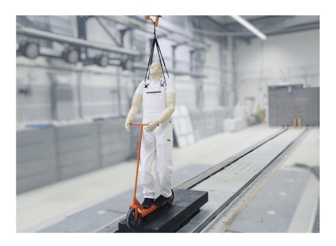
In the crash tests, the e-scooter and dummy were driven against a curb at speeds of 10, 20 and 30 km/h. Even at 10 km/h, there is a significant risk of injury. Credit: Fraunhofer EMI
