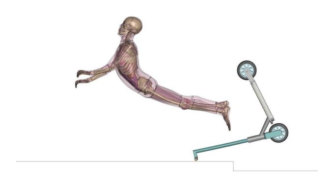
The moment shortly after impact in the simulation. The human model is catapulted into the air over the handle-bars. Credit: Fraunhofer EMI
