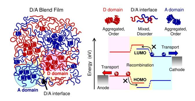
The high FFs (~70%) of the all-polymer blend solar cells were achieved because of the longer charge-carrier lifetimes due to the lower bimolecular charge recombination coefficients. The preferred blend morphology for suppressing the bimolecular charge recombination is characterized by a well-ordered local structure due to chain aggregation by both the polymer donor (D) and acceptor (A). Credit: Hiroaki Benten
