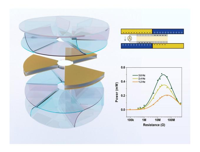
This diagram shows the schematic of the constant inherent capacitance triboelectric nanogenerator, the working mechanism of the device with two surfaces rubbing against each other, and the output powers of the device. Credit: *Nano Research*
