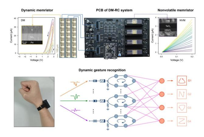
Figure summarizing the hardware architecture and application of the DM-RC system. Credit: Zhong et al.
