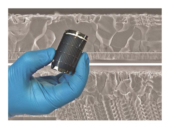
Flexible CIGS solar cells are composed of very thin layers, including a compound composed of the elements copper, indium, gallium and selenium. The layers are deposited onto flexible polymer substrates, mainly by vacuum processes. Credit: Swiss Federal Laboratories for Materials Science and Technology
