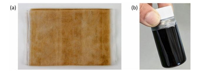
a) Photograph of a section of face mask material used for CNT production. Sections were cut and b) dispersed in toluene to form the plastic carbon precursor seen in a vial. Credit: *Carbon Letters* (2022). DOI: 10.1007/s42823-022-00398-8
