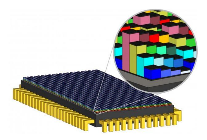
HSI chip with per-pixel filters forming a 4x4 pixel mosaic. Credit: IMEC
