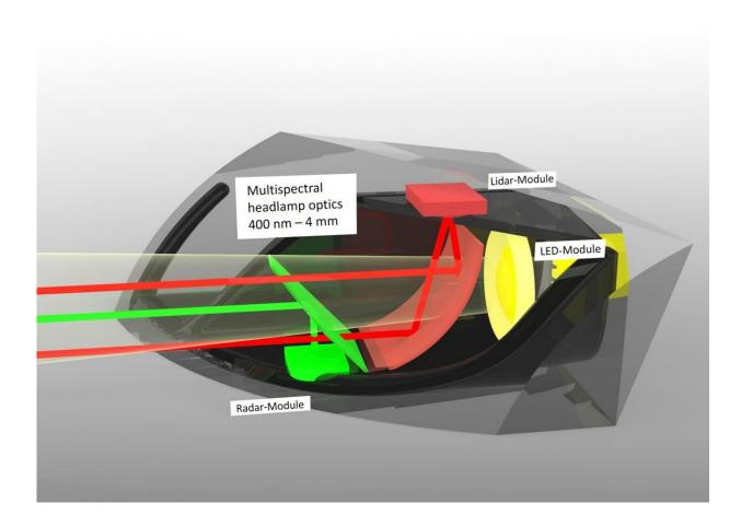
LED headlight model with multispectral combiners for coaxially merging optical light, LiDAR (red) and radar beams (green), with the aim of achieving spacesaving sensor integration for next-generation driver assistance systems. Credit: Fraunhofer FHR
