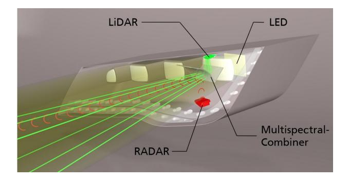
3D visualization of multi-spectral headlight optics. Credit: Fraunhofer FHR
