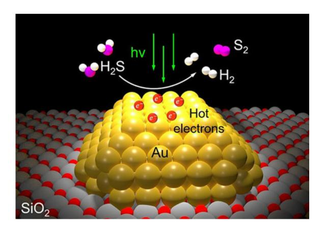
An illustration of the light-powered, one-step remediation process for hydrogen sulfide gas made possible by a gold photocatalyst created at Rice University. Credit: Halas Group/Rice University
