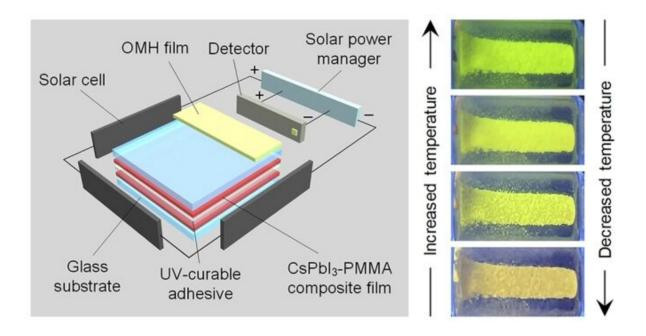
The temperature alarm system is self-powered by luminescent solar concentrators based on a single green-emitted PEA2MnBr2I2 with a backward energy transfer process. Credit: *Journal of Energy Chemistry* (2022). DOI: 10.1016/j.jechem.2022.09.036
