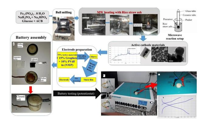
Synthesis process of sodium iron phosphate through ball milling and microwave assisted and assembly of related batteries and supercapacitors. Credit: *Scientific Reports* (2022). DOI: 10.1038/s41598-022-20329-x
