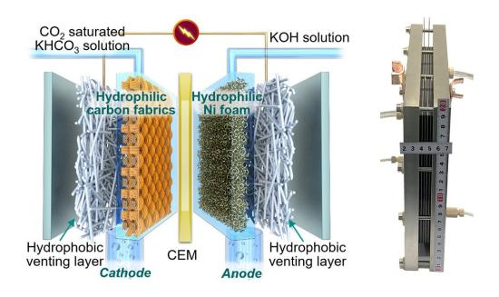
Left: a schematic showing the key components of the reactor and working mechanism. Right: a picture of the  $CO_2$  stack, which is a demonstration of the commercial reactors. Credit: Dr. Zhongwei Chen, a chemical engineering professor at the University of Waterloo
