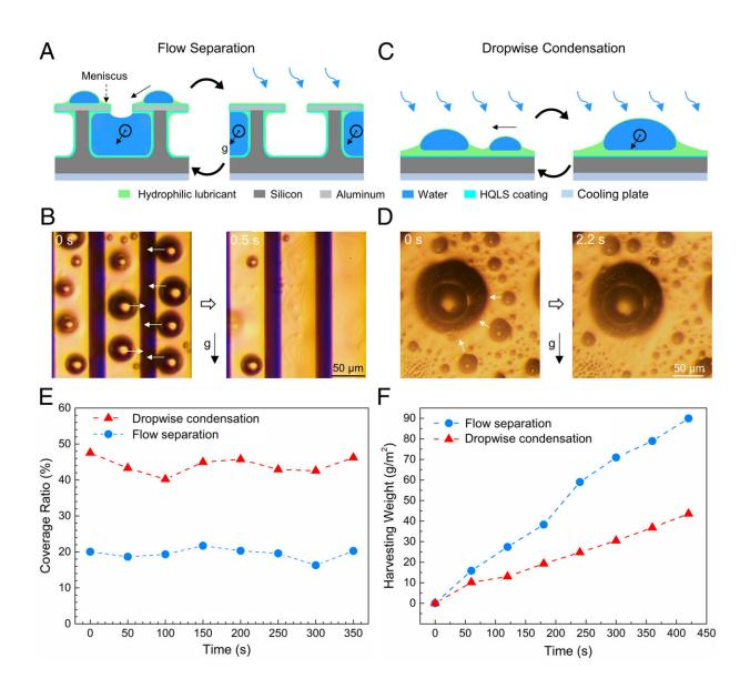
Flow separation on hydrophilic reentrant SLIPS. (A) Schematic of flow separation. The small droplets move into the reentrant channels due to
