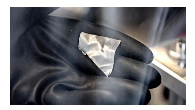
In the laboratory, lithium is kept in a glove box because it reacts with the oxygen, water and CO2 in the air around us. The box contains pure argon gas. The oxygen and water content in the box is 0.1 parts per million. Credit: Bax Lindhardt
