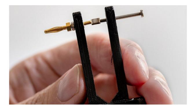
The only commercially available rechargeable solid-state battery on the marked is used in microelectronics. It supplies the device with power when it is not connected to a power outlet. Here in the laboratory, it is mounted in a device that lets the researchers conduct X-ray diffraction while the battery charges and discharges. Credit: Bax Lindhardt
