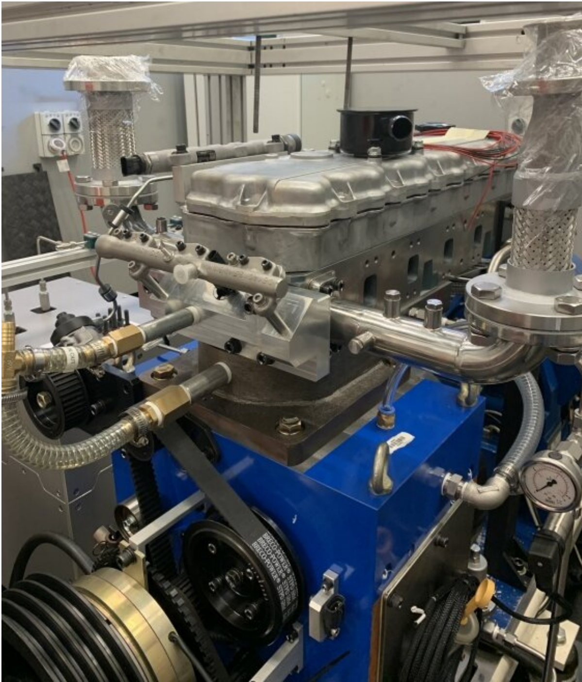
The hydrogen-diesel direct injection dual-fuel system developed at UNSW enables a traditional diesel engine to be retrofitted to run as a hydrogen-diesel hybrid engine. Credit: Prof. Shawn Kook
