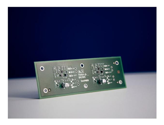
Test PCB with functional structures for generating a digital fingerprint. Credit: Fraunhofer IZM
