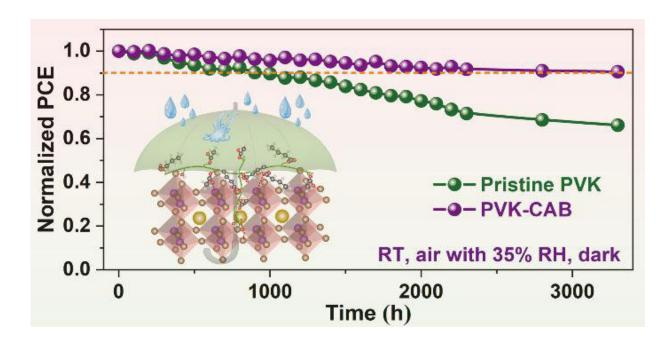
Functional groups of cellulose acetate butyrate (CAB) interact with anions and cations in perovskite (PVK) to significantly improve the device stability by inhibiting the decomposition of perovskite. Credit: Journal of Energy Chemistry
