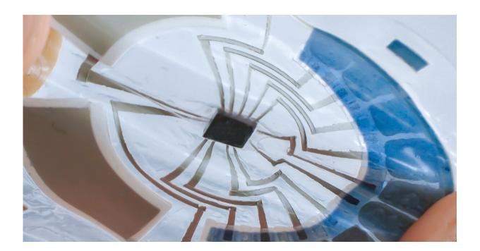
This stretchable patch includes a display panel, battery, sensor and microcontroller. Credit: Lu Yin, Jacobs School of Engineering, UC San Diego.
