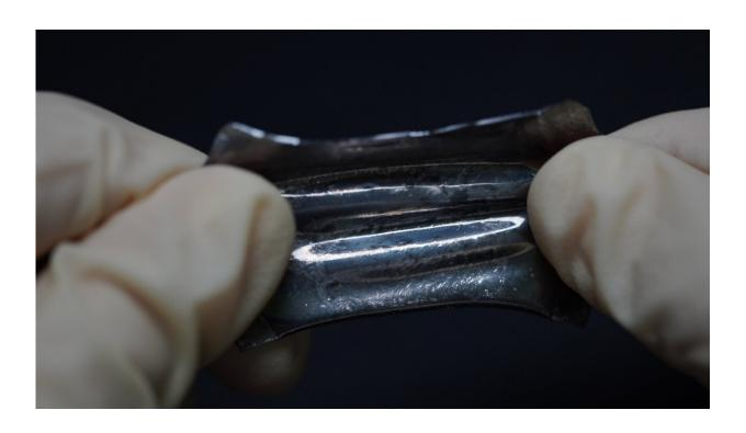
Stretchable battery which is packed in liquid metal is strained by hands. Batteries can withstand stretching of more than 50%. Credit: Yokohama National University
