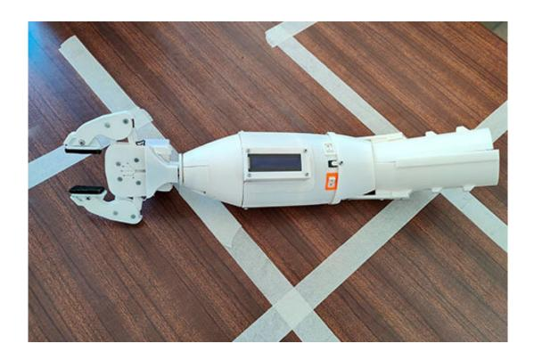
Detail of the 3D-printed transradial myoelectric prosthesis. Credit: Polytechnic University of Catalonia
